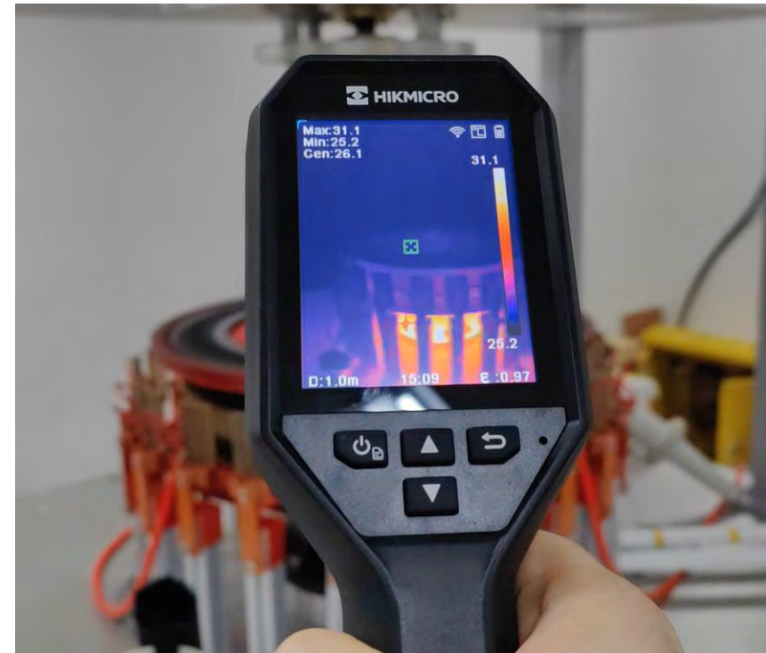
Thermovision camera HIKMICRO. MEC rollers temperature after 60 minutes of work
