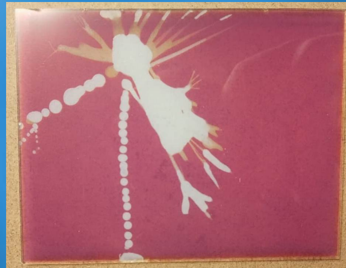
Up. A trace in the form of a «girl in a dress» on an X-ray sensitive glass plate 9 \times 12 [cm 2 ], 1.4 [mm] thick.
