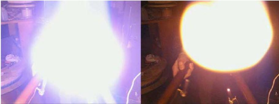
Volumetric discharge with carbon electrodes accompanied with combustion and its afterglow
