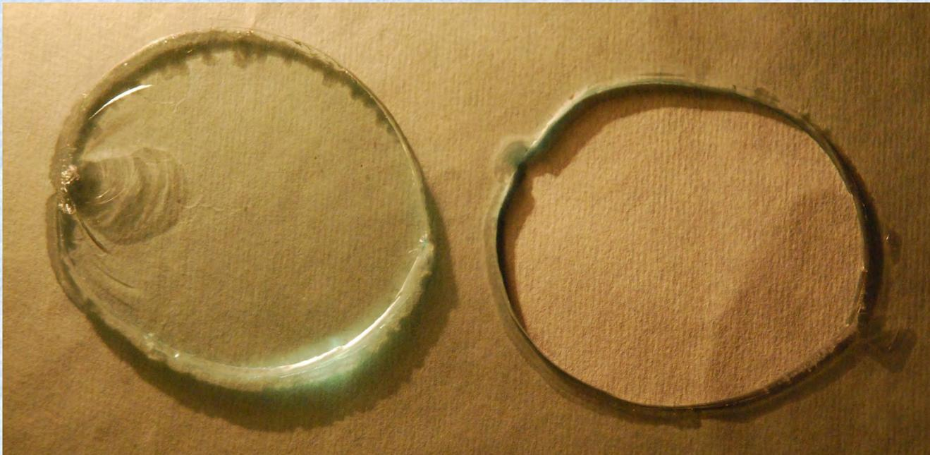
To the right is a hole in the glass, to the left is the disc that had fallen out the hole. Disc (hole) axes sizes are 8.2 and 7.6 cm.
