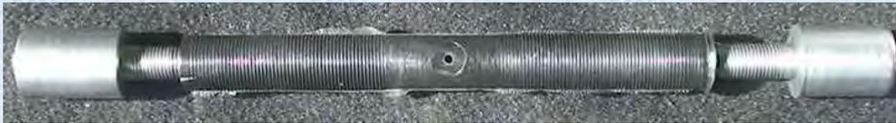
Electrodes with the polymeric pipe
